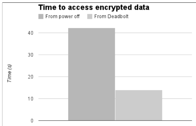
(a) Average time to access encrypted data from power off and from Deadbolt.
